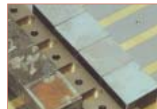
Number of small components can be machined using simple pole extension fixtures.
