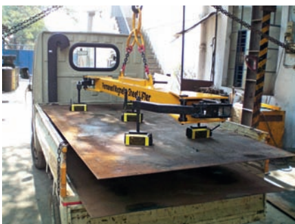
Spreader Beam With Adjustable Magnets.
