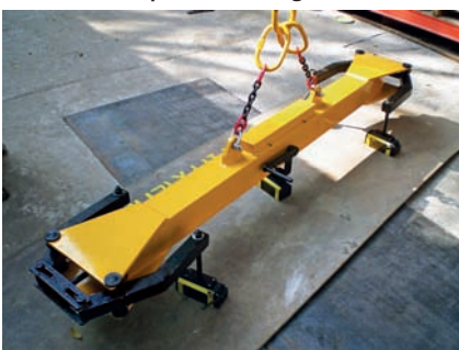
Spreader Beam With Adjustable Magnets.
