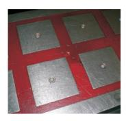
When different materials are used in the top face, due to heating and damage there is a chance of seepage of coolant/ liquid into the chuck, which results in burning of coil. Repair of coil is difficult, as no repair can begin without first destroying the chuck.
