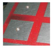
Due to heavy machining there is unequal heating of steel and epoxy resulting in inaccuracies and damage to surface. As the working face is made of single monolithic block of steel, inaccuracies due to unequal heating is reduced and there is no damage to the surface.
